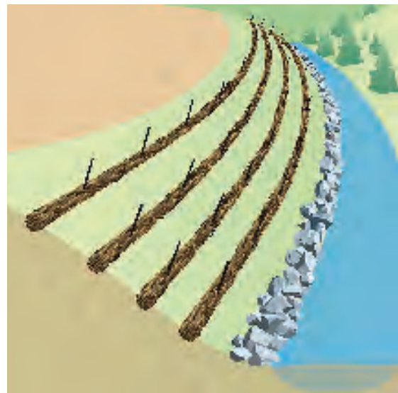
Coconut logs, fiber rolls, and other products can be used in conjunction with wattles to ensure adequate protection while plant material is becoming rooted. Follow manufacturer's installation information.
