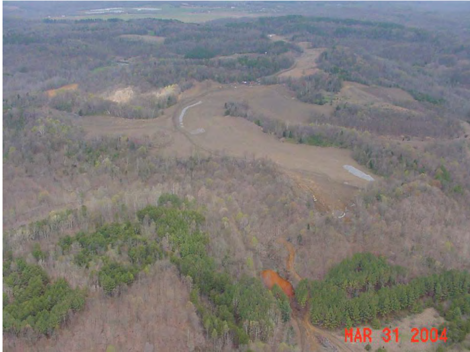
Figure 14: Main site after agriculture limestone barrier and earthen cover application.
