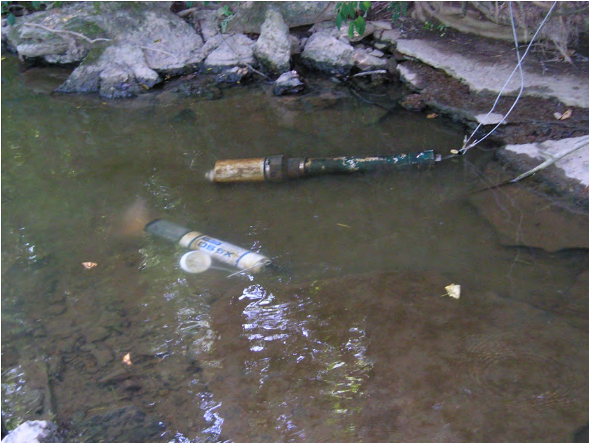
Figure 6. Photograph of continuous monitor deployed at the Frog Branch monitoring station FB1 with QA/QC monitor .
