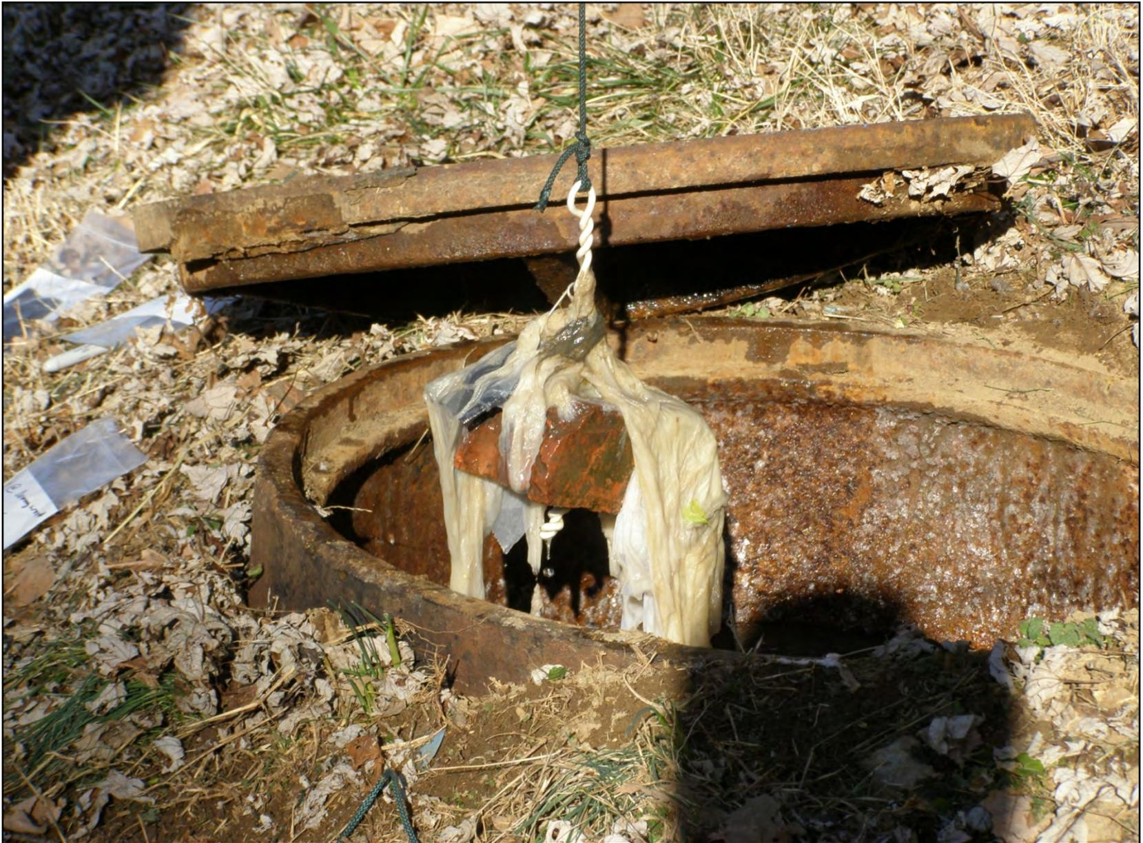
Figure 35a. Inconsistent Dye Monitoring in Sanitary Sewer with Dye-Receptor Submerged on Brick Anchor following 1 hour of deployment and covered with sewer solids
