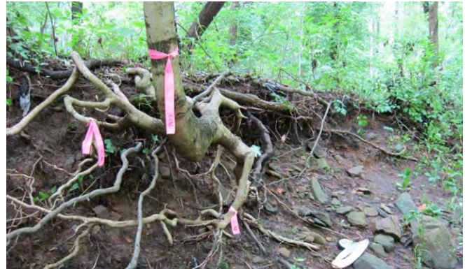
Figure 2.5b Upright tree measurement, L, used to calculate lower limit of erosion rate.
