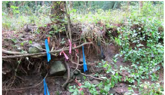
Figure 2.5d Root-with-sucker measurement, L, used to calculate a lower limit of erosion rate.
