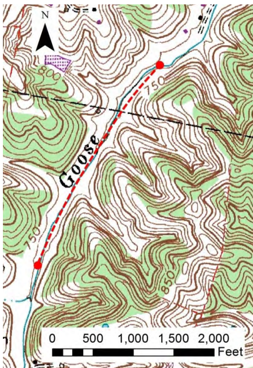
Figure C.2 An approximate measure of valley slope can be made from contours on a USGS topographic map.
