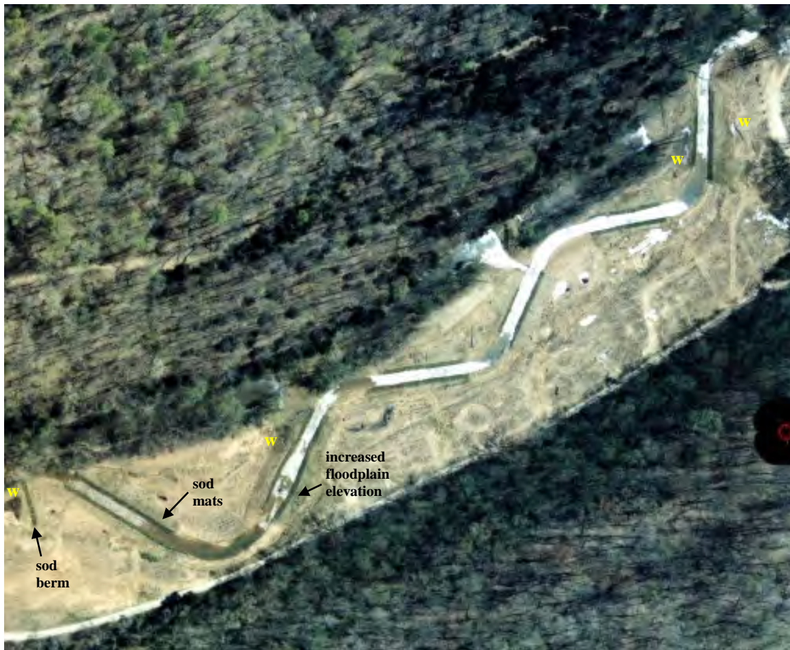
Figure 3 Aerial photo showing elements of floodplain and channel changes (downstream section of restoration). The letter "w" indicates a location of a wetland created during the enhancement project.
