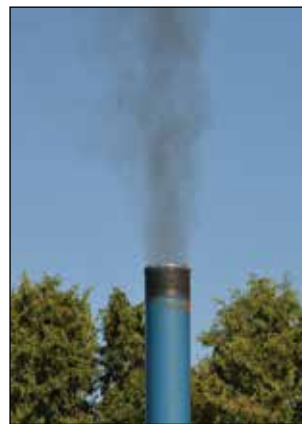
TOP: Smoke School students observe visible emissions plumes to identify opacity levels of smoke. ABOVE (left to right): Black smoke at opacity levels of 25 percent, 50 percent and 75 percent are used during Smoke School to calibrate an observer’s eyes.
