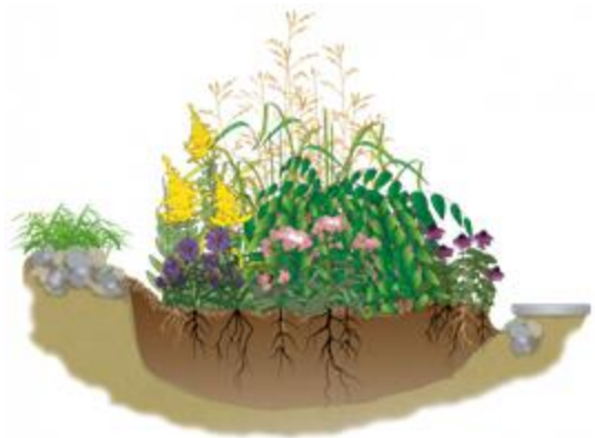
Above is a picture of a rain garden to minimize storm water runoff
