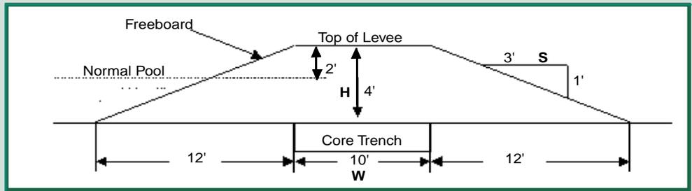
Figure 1. Cross section of a typical levee with a 3:1 slope.
