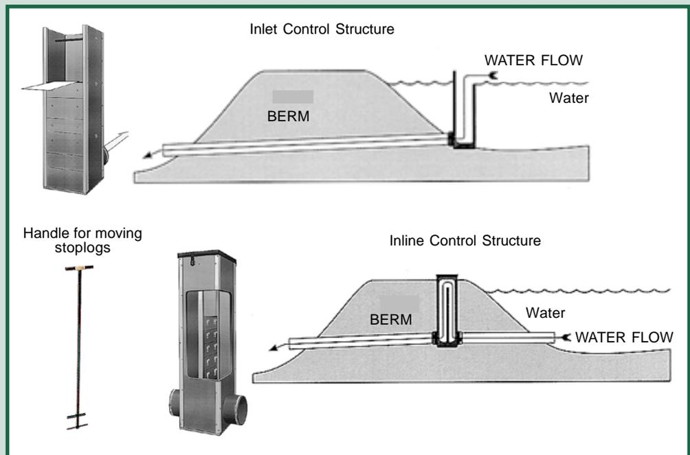
Figure 3. Prefabricated inlet and inline box type flashboard risers. Web site images courtesy of Agri Drain Corporation at [www.ad-copr.com](http://www.ad-copr.com)
