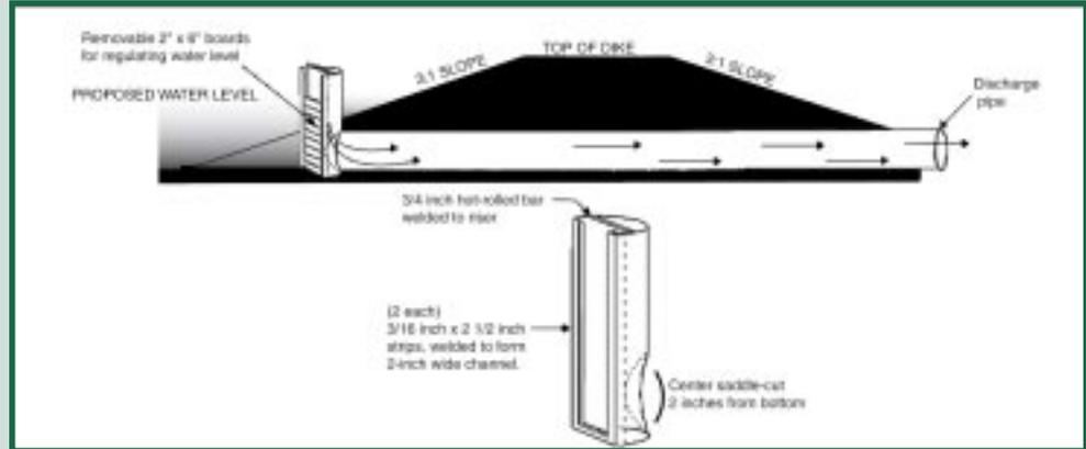
Figure 2. Half round flashboard riser inlet water control structure constructed from steel pipe. Reprinted from *Waterfowl Habitat Management Handbook for the Lower Mississippi River Valley*, Ducks Unlimited, Inc. 1993
