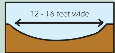
Figure 6. Side view, showing change in pond grade.
