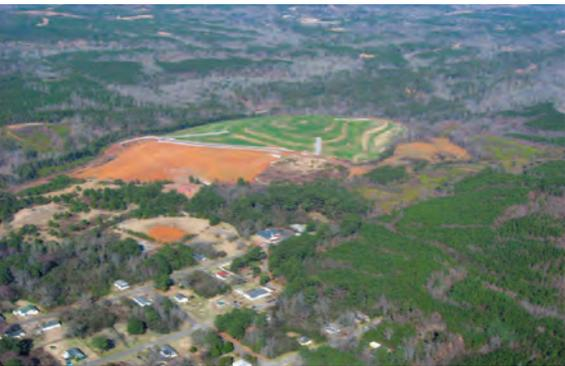
Reclamation was accomplished by separating the burning material and sealing lifts with clay, effectively separating the fire from its source of air. Once graded, riprap down-drains, revegetation and tree planting successfully stabilized the site. Including borrow and disposal areas, the final project footprint included 52 acres at a cost of \$2,731,000.
