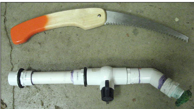
The hand saw (top) and the herbicide wand (bottom) provide a light, inexpensive way to treat new infestations in the backcountry. Jack McGowan-Stinski of The Nature Conservancy designed the wand. For info on building your own wand go to: http://tncweeds.ucdavis.edu/tools/wand.html ~ Andrew Berry, KSNPC
