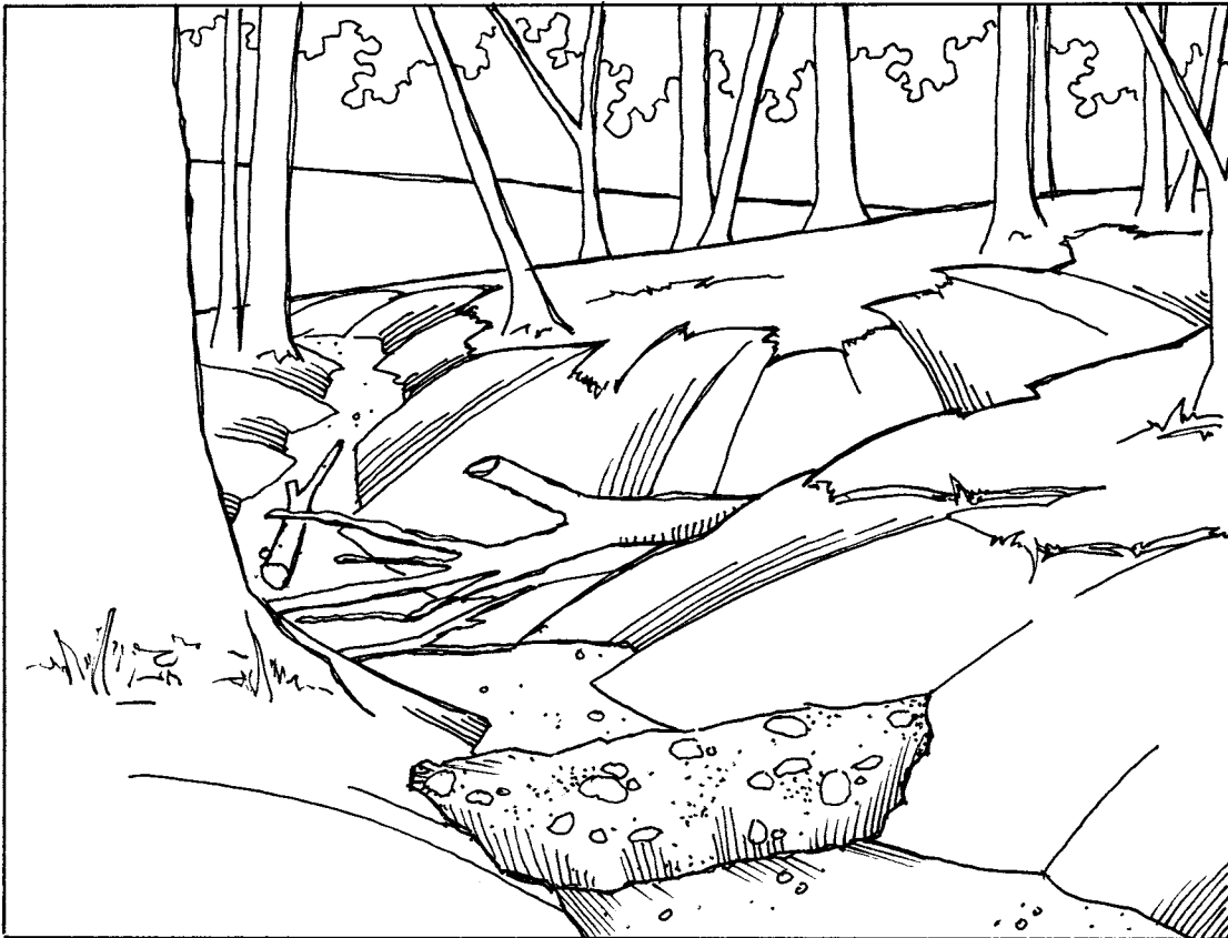
Figure 17. Woody debris and gravel bar used to slow erosion and discourage continued trail use
