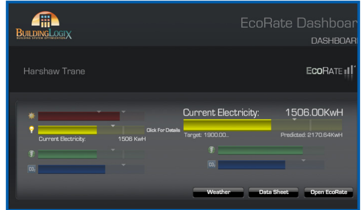
Utility meters are connected to an electronic, web-based energy dashboard, like this one, where the data is displayed on a monitor in a central location.
