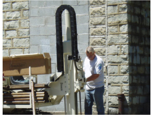
Superfund employee Mike Blanton uses a geoprobe to take soil samples at a property in Wheelwright, Ky.
