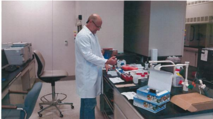
Gerry Morford (Technical Services Section – Environmental Scientist V) loads an ELISA plate counter for HAB - Microcystin analysis.
