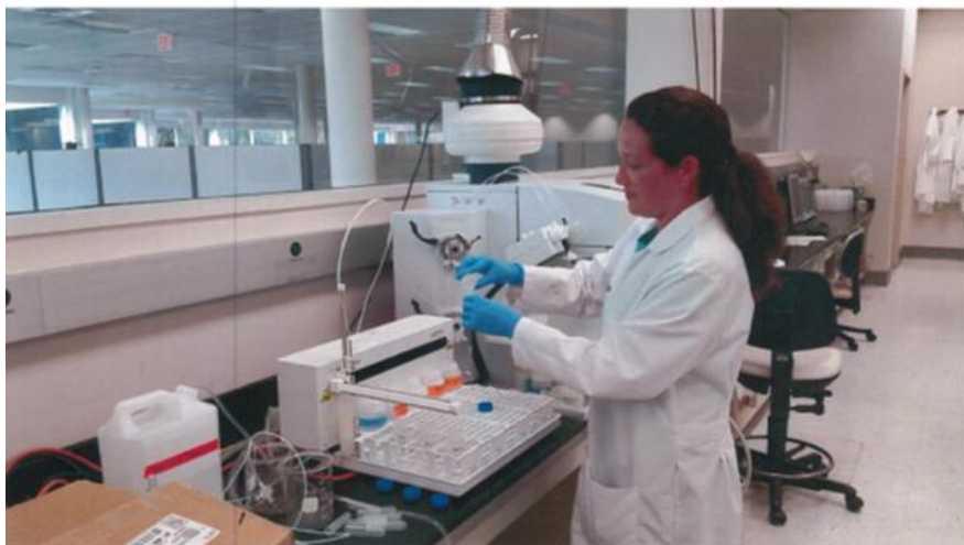
Shannon Dutta (Metals Section Supervisor) loads samples onto an Inductively Coupled Plasma Mass Spectrometer (ICPMS) auto sampler.
