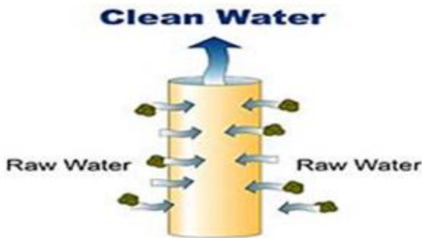
Above: A strand of membrane in action Below: A cassette housing membranes
