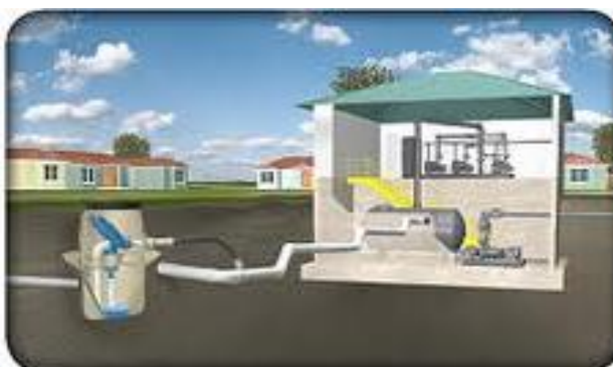
Picture 4-12 Vacuum system in home connection diagram
