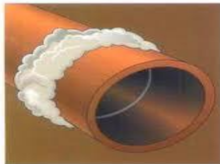
Picture 11-7 Grouting on the exterior of a pipe
