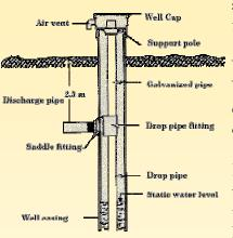
surface while providing a watertight seal, which prevents bacteria and soil fauna from getting into your well (see the diagram to the left).
