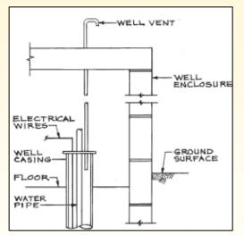
Figure 4. Recommended venting procedures for wells located in enclosed structures.
