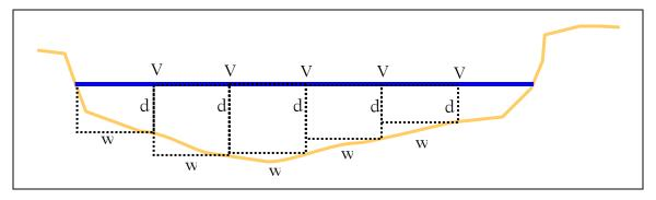
Stream cross-section showing intervals where water depth and velocity are measured. Flow will be calculated for each "box" (flow area for each box is d \* w) and summed to obtain the flow for the entire stream.
