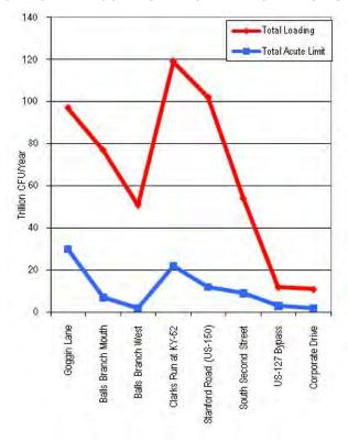
To calculate watershed reach specific loadings, the total loadings of upstream stations are subtracted from downstream sites. This reach specific loading provides a better indication of the geographic sources of load inputs. The loadings for each reach, and the reach specific reduction goals are shown in Table 20 and Figure 6.
