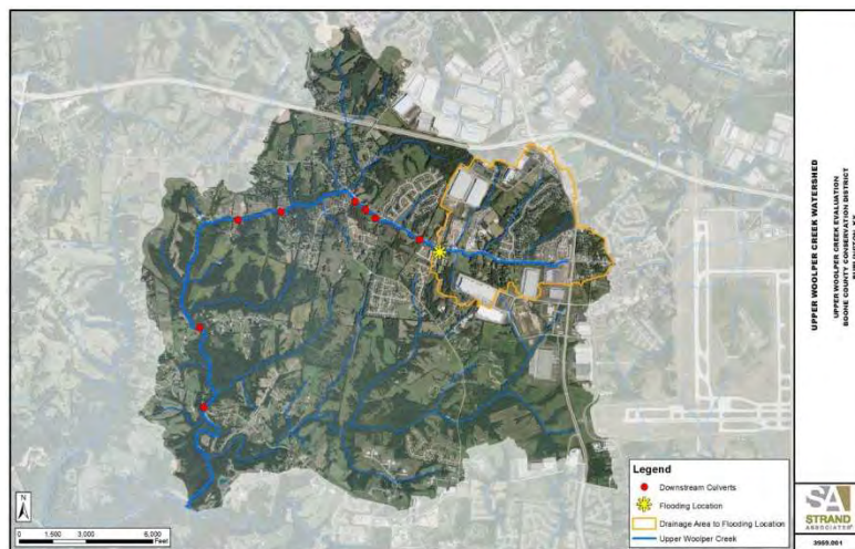
Figure 5-11: Flooding location in the headwaters of the Upper Woolper Creek Subwatershed provides focus for detention basin retrofit study upstream
