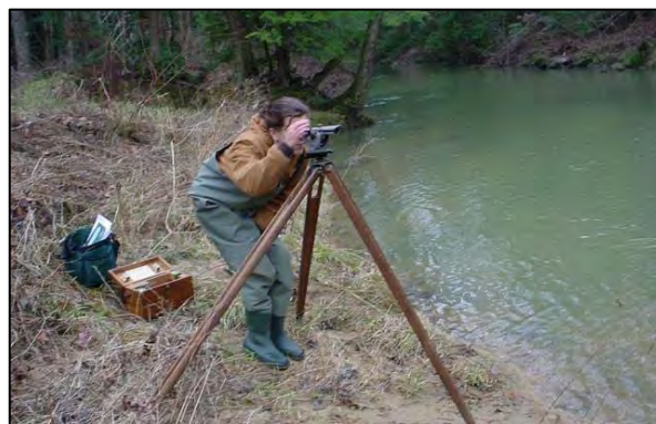
Surveying Stream Cross Section
