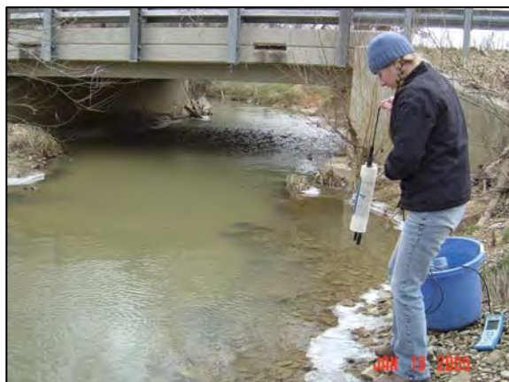
Using Hydrolab probe to measure stream pH, conductivity, dissolved oxygen, and temperature during a pedestrian survey, Site 15B
