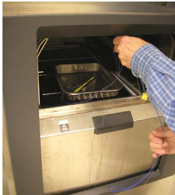
Figure 5. Method of closing autoclave door on the thermocouples.
