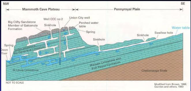
**Figure 86.** The Ste. Genevieve and the St. Louis Limestones that underlie the Mammoth Cave Plateau contain a well-developed network of solution openings. These openings were formed by dissolution of the limestones as ground water moved along bedding planes and fractures from recharge areas to points of discharge.
