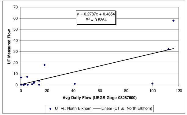
Figure C.3 Correlation between Measured Flows at Site 04NE of UT to Upper North Elkhorn Creek and Average Daily Flows at the USGS Gage
