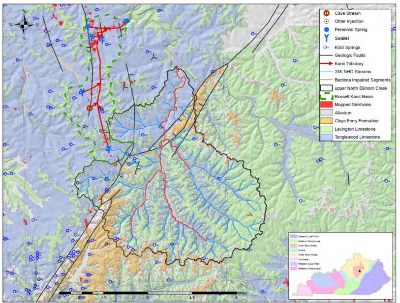
Figure 3.1 Geologic Map of the Upper North Elkhorn Creek Watershed Demonstrating the Presence of Mapped Faults and Karst Features
