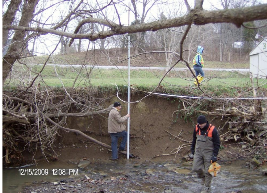
Figure 3 – Highly Unstable Bank Experiencing Mass Wasting (Site TUC0.4 – Right Bank Index = 0)
