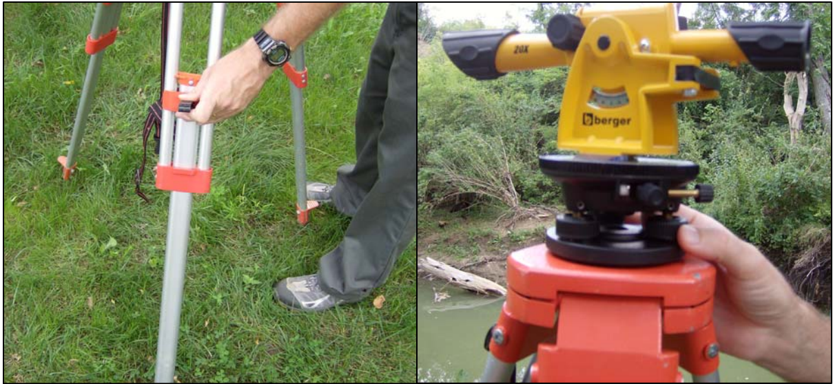
Figure 3. Adjust the legs and fine adjustment knobs to make the instrument level.
