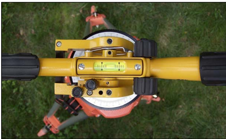
Figure 4. The instrument is level when the bubble remains centered at any orientation along the 360^\circ circumference.
