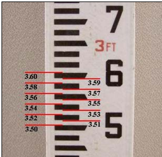
Figure 6. To get a measurement, first determine the ones place on the rod by locating the red number. The tenths place is the larger number on the right of the rod. The hundredths place is either on the top or bottom of each line.
