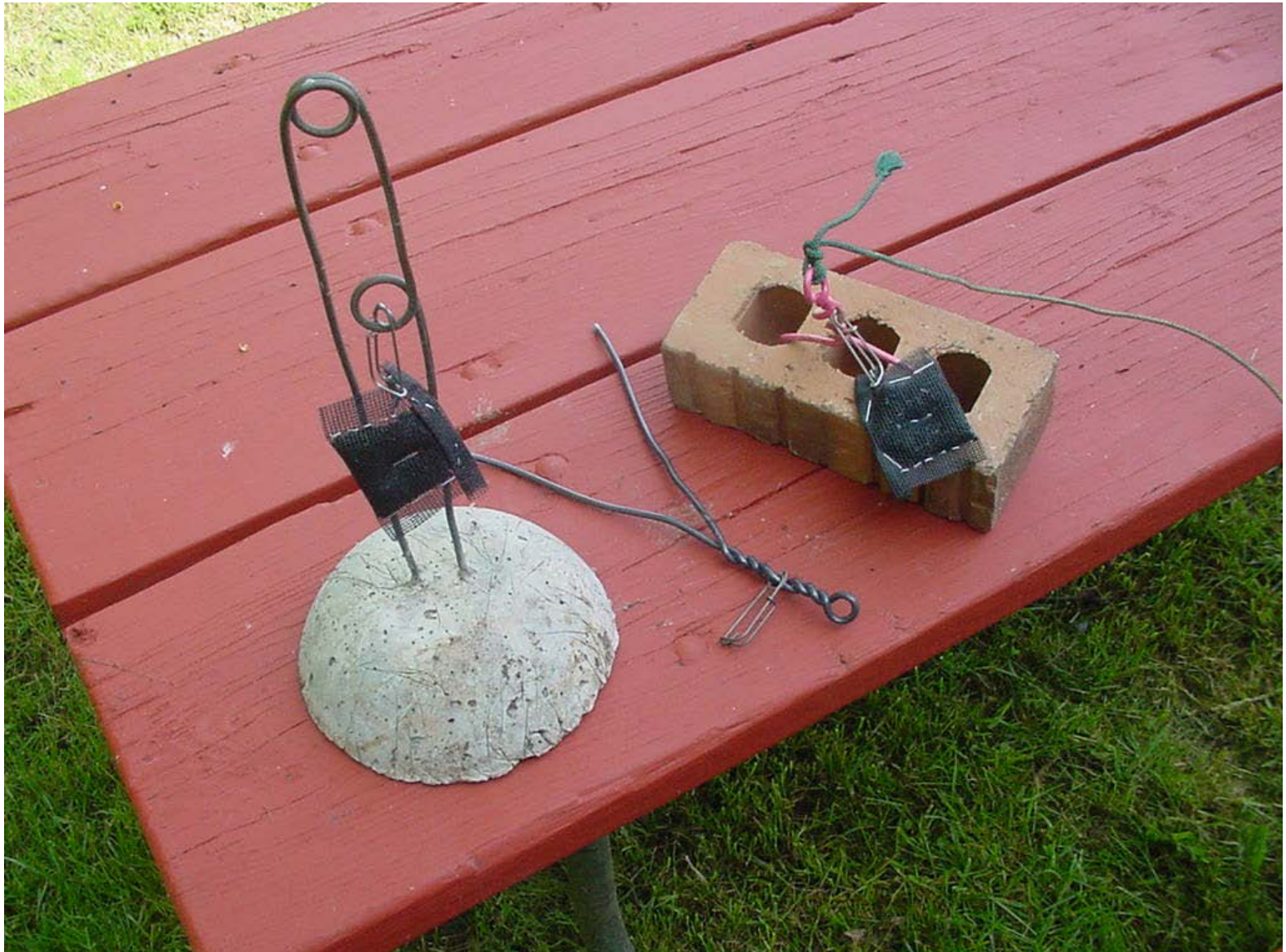
Figure 6. Activated charcoal packet attached by trot-line clip to “Quinlan Gumdrop” or brick fitted with #10 copper wire. Devices secured to retrieval point with nylon cord.
