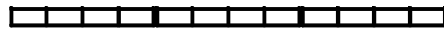
FIG 1. PLACE A ROW OF CONSTRUCTION FORMS ALONG DESIRED CHANNEL ALIGNMENT FOR FIRST LIFT.
