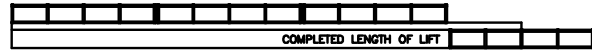
FIG 2. CONSTRUCT FABRIC WRAP LIFTS ALONG LENGTH OF FIRST SET OF FORMS AND THEN BEGIN PLACEMENT OF FORMS AND CONSTRUCTION OF SECOND LIFT.
