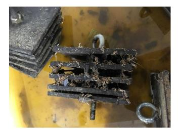
Figure 6. Hester Dendy unit after colonization period showing variable spacing between the hardboard plates.
